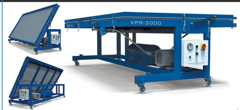
The VPR is a cold membrane vacuum press is designed for woodworking and furniture production. Membrane press is equipped with rotary work-table, which saves production space and allow use it in small workshops. The vacuum press can be supplied in two ways: as fully equipped vacuum press VPR-3000/25 or VPR-3000/40 and as vacuum table VPR-3000T (without vacuum system).
